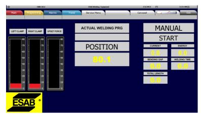
· The programming phase is an easy-to-learn easy-to-use procedure starting with the adding of wished modules (pre-flashing, pre-heating, flashing and upsetting). Later every module will be "opened" in order to set the parameters and choose the working modes.
