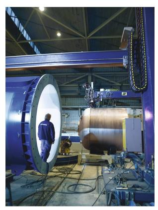
Among other things, the upgrade has involved switching from single to twin wire, thereby improving the deposition rate. In addition, a new flux system has been installed and the continuous supply reduces stoppages caused by the necessity of filling up with flux. The new welding equipment has also created conditions for more reliable production with less downtime.
