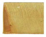
When compared to Nitrogen Plasma or Argon-Hydrogen Plasma, Water Injection cutting creates a smoother, cleaner edge finish with minimal dross and less heat-affect zone.
