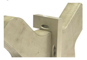
Water injection plasma cutting of stainless steels and aluminum alloys offers exceptional cut quality including a highly desirable cut edge surface with little or no dross.
